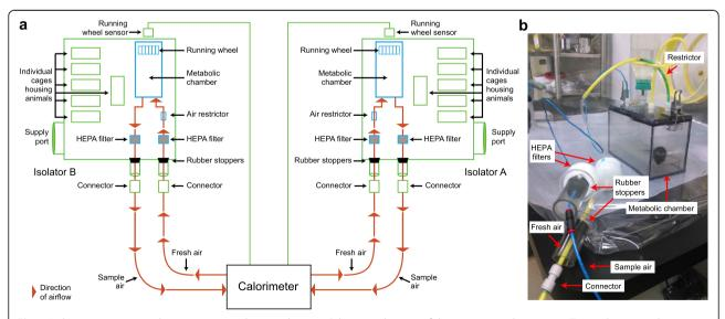
**Fig. 1** Indirect open-circuit calorimetry in gnotobiotic isolators. **a** Schematic drawing of the experimental apparatus. Two isolators are shown: isolator A contains animals colonized with bacterial consortium A from the lean co-twin; isolator B contains animals harboring bacterial consortium B from the obese co-twin. **b** Photograph of flexible film gnotobiotic isolator containing a metabolic chamber and devices used to connect the chamber to the exterior calorimeter
